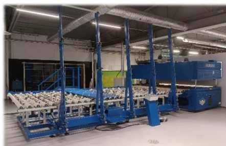
Newly installed digital printer Vitro-Jet FC Type and rest of machines in-line of the complete Turn-Key solution at Forserum Safety Glass AB
