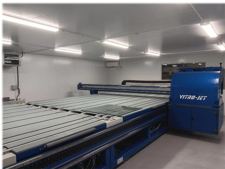
Newly installed digital printer Vitro-Jet FC Type and rest of machines in-line of the complete Turn-Key solution at Forserum Safety Glass AB
